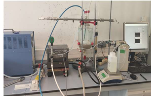
RO bench scale experimental set-up
