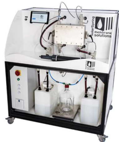
MD bench scale experimental set-up
