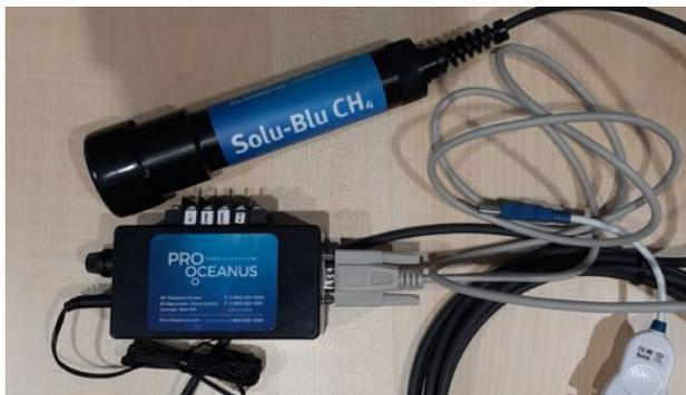
Gas sensors and dissolved methane probe to assist on the measurement of energy production in the AnMBR
