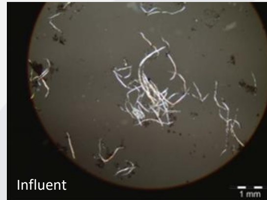
Visible reduction of fibers in raw influent
