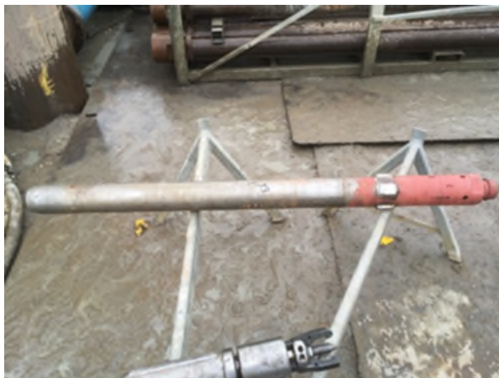
Figure 26. Picture of the coring device that was used to obtain the core samples.
