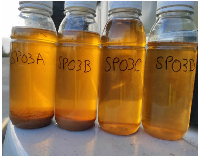
Figure 108. Samples collected from the different sections of the reactor A to D, from bottom to top.
