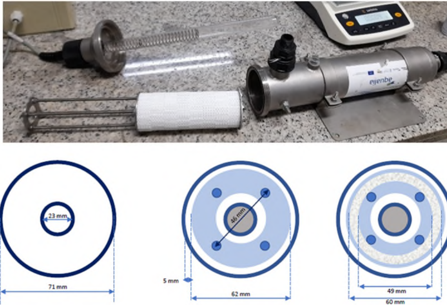
Figure 62. Top: photocatalytic reactor with support and first (white) PLA prototypes. Bottom: three sections of the UV lamp, where toroidal structures can be inserted.
