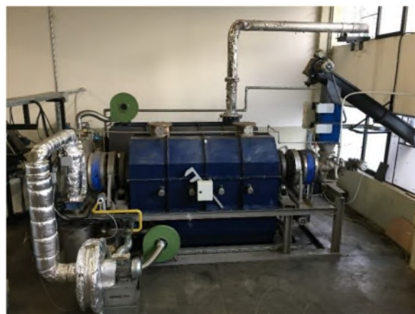
Figure 36. Rotary kiln for slow pyrolysis (PYROCK).
