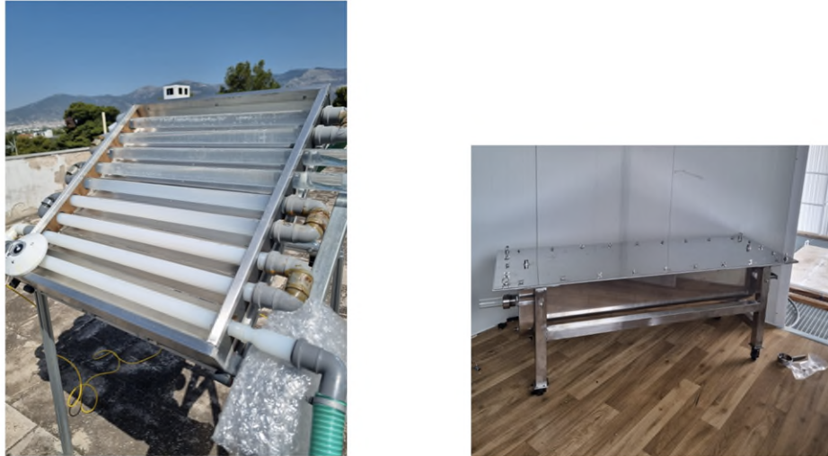
Figure 47. CS4 photocatalytic reactor.
