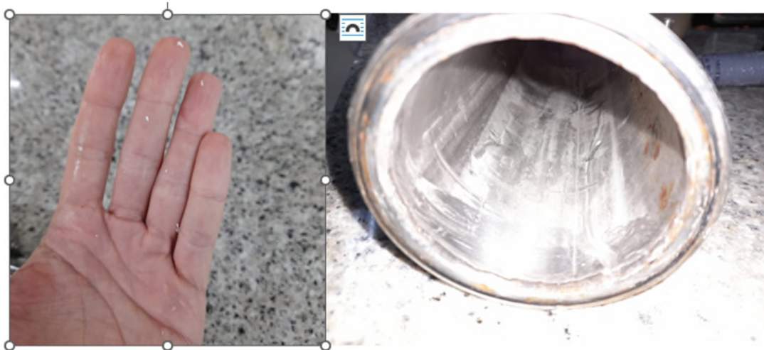
Figure 78. Some thermoplastic particles and dust were observed after first Aqualia's tests, proving that resistance of the structure had to be improved, although the reasons of these damages were not fully understood. Samples were sent to the CSP supplier.
